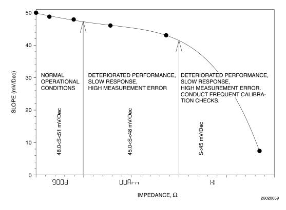
Figure 6-1. Slope vs. Impedance
